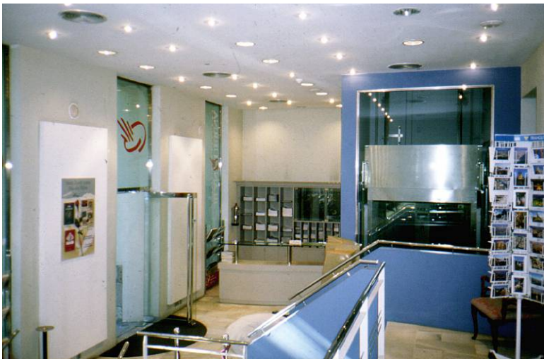
Fig. 11 and 12. The correct use of an elevator allows solving complex situations. This building that lacks space at the street level, gains access to the attic and semi-basement by a double-door elevator.
